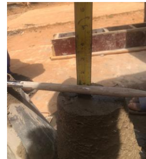
Figure 3.2: Measurement of slump value for sample A
