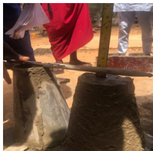
Figure 3.3: measurement of slump value for sample B
