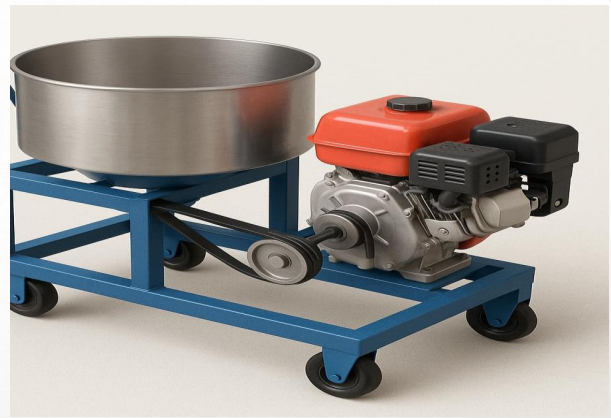
Fig. 4.1: A labeled 3D representation of the complete machine showing the bowl, frame, motor, and castor wheels.
