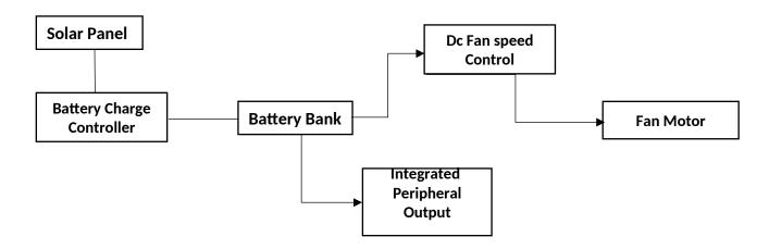
Figure 3.1 Assembling block diagram
