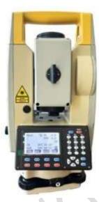
The instrument is used to measure sloping distance of object to the instrument, horizontal angles and vertical angles. This Microprocessor unit enables for computation of data collected to further calculate the horizontal distance, coordinates of a point and reduced level of point.
