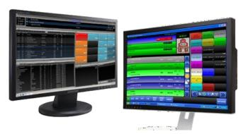
The computer system that plays back music, spots (ads, promos, etc.) and sweepers(the little voice-overs played between songs) is called a Play out System or Automation Software. These are specially designed computer programs that allow for continuous playback of audio, with a lot of granular control for Announcers and Programme Directors.
