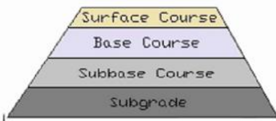
Fig 1. Section of Flexible Pavement
