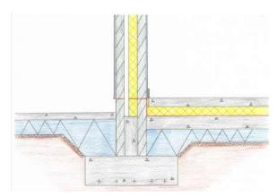
2. Pad Foundation: A square or rectangular concrete pad used to support a column.
