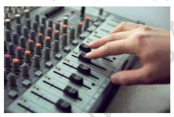
There are analog audio consoles and digital audio consoles, but radio consoles, in general, are specifically designed to be easy for on-air talent to use. In an analog console, the physical audio is actually transmitted through its circuitry. In contrast, digital audio consoles function as a "remote control" for the mix engine (typically located within the rack room).
