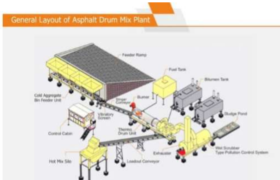
General layout of Asphalt drum mix plant
