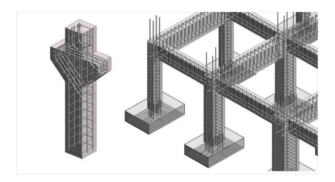
After the reinforcement then would be a framework which will be at the outer part of the reinforcement to guide the casting of the column.
