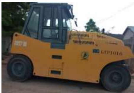
Pneumatic rubber tyre roller
