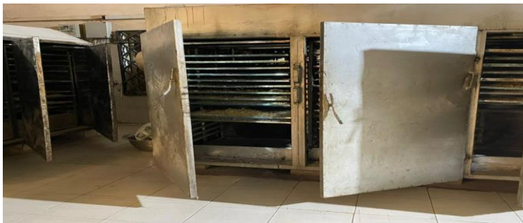
Fig 3.5: An industrial cabinet dryer
