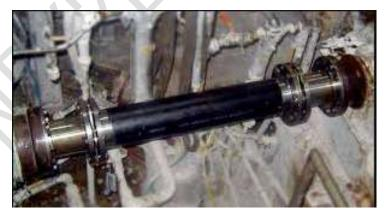
**3. Parallel misalignment** occurs when two shafts are parallel to each other but not in the same plane, meaning they are offset from each other. This can happen horizontally or vertically.
