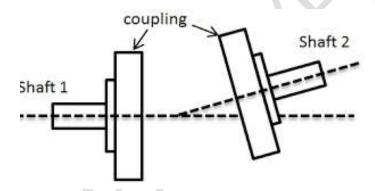
**8. A flexible coupling** is a mechanical element that connects two shafts, allowing for some degree of misalignment and accommodating movement, vibrations, and shock absorption while transmitting power and movement.
