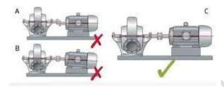
**7. Angular misalignment** occurs when the axes of two connected shafts intersect at an angle, rather than being parallel, leading to potential problems like increased vibration and premature wear of components.
