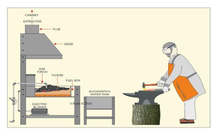
Blacksmithing involves the manipulation of heated metals to achieve specific shapes and forms. The Forging Section focuses on the art of forging, where metals are heated and hammered into desired configurations. This section not only imparts practical skills but also fosters an appreciation for the historical significance of blacksmithing in the evolution of metallurgy.
