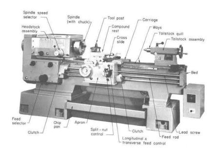
The Lathe Machine is a versatile tool in metallurgical workshops, enabling students to perform precision turning and shaping of metals. Its application ranges from creating cylindrical components to intricate machining tasks. Students learn to operate the Lathe Machine, gaining proficiency in metalworking techniques that are fundamental to various mechanical processes.
