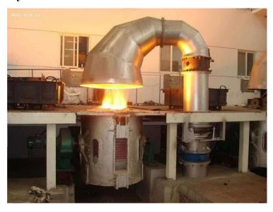
The Hydro Lift Out Crucible Furnaces stand as a cornerstone in the metallurgical processes conducted within the Mechanical Engineering Department. These furnaces play a vital role in the melting and casting of metals, offering students hands-on experience with the intricate procedures involved. The furnace's design allows for precise control of temperature and facilitates the safe handling of molten metals, contributing to a comprehensive understanding of metallurgical principles.
