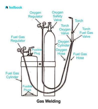
Gas welding is a foundational skill in metallurgical engineering, and the Gas Welding Machine serves as a primary tool for students to develop proficiency in this area. Through practical exercises, students gain hands-on experience with gas welding techniques, safety protocols, and the intricate art of joining metals using this versatile equipment.
