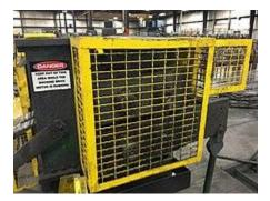
Point guarding around gear operation of machine
