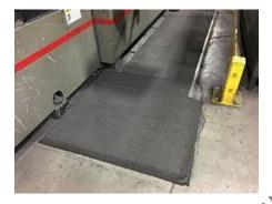
Pressure sensitive mat for operator of laser cutter
