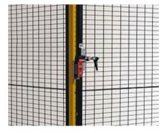
Electrical interlock mounted on wire mesh machine guarding
