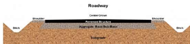
Plate 1.0: Road cross section
