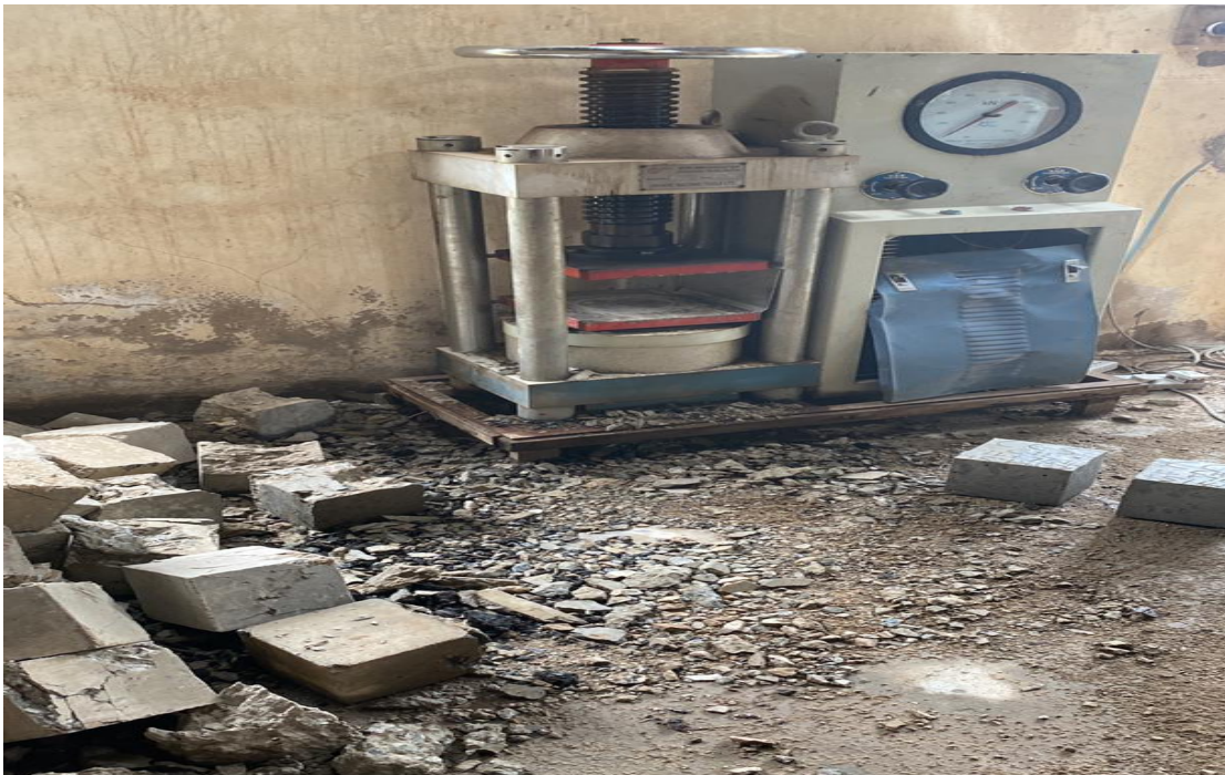
Figure 4.5: Compressive testing machine and crushed Cubic Concrete Sample.
