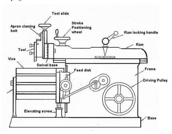
In the arsenal of mechanical machinery, the Shaping Machine stands out for its ability to shape and form metal workpieces with precision. Students engage with the Shaping Machine to understand the principles of metal shaping, honing their skills in creating components with specific geometries and dimensions.
