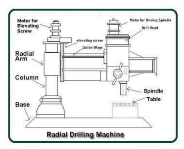
The Drilling Machine is a fundamental tool in metallurgical workshops, facilitating the creation of holes in metal workpieces. Students learn the intricacies of operating the Drilling Machine, mastering techniques such as hole positioning, depth control, and selecting appropriate drill bits for various materials.
