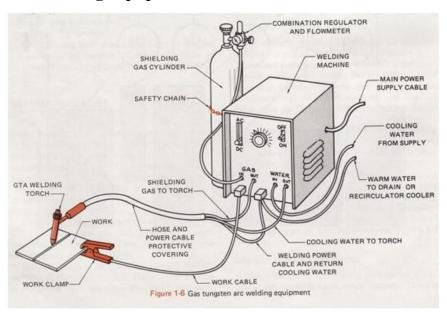
Arc welding is a cornerstone technique in mechanical engineering, and students are exposed to various types of Arc Welding Equipment. This includes welding machines that utilize different types of electrodes and welding processes. Through hands-on exercises, students acquire skills in arc welding, contributing to their ability to perform precision metal joining and fabrication.
