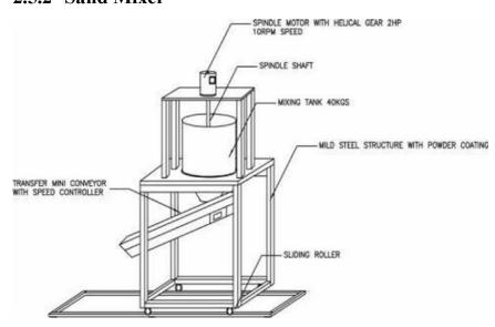
The Sand Mixer is a key component in metallurgical processes, especially in the preparation of molds for casting. Students engage with the Sand Mixer to understand the intricacies of sand preparation, a fundamental aspect of ensuring the quality and integrity of castings. The hands-on experience with the Sand Mixer connects theoretical knowledge with practical application, emphasizing the significance of proper mold preparation in metallurgical engineering.
