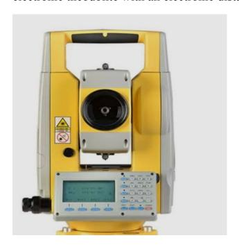
**2. Theodolite:** A precision instrument for measuring angles in horizontal and vertical planes. It is commonly used in triangulation and leveling work. A theodolite uses a movable telescope to measure angles in both the horizontal and vertical planes.
