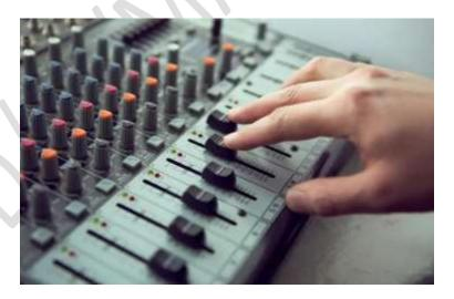
There are analog audio consoles and digital audio consoles, but radio consoles, in general, are specifically designed to be easy for on-air talent to use. In an analog console, the physical audio is actually transmitted through its circuitry. In contrast, digital audio
