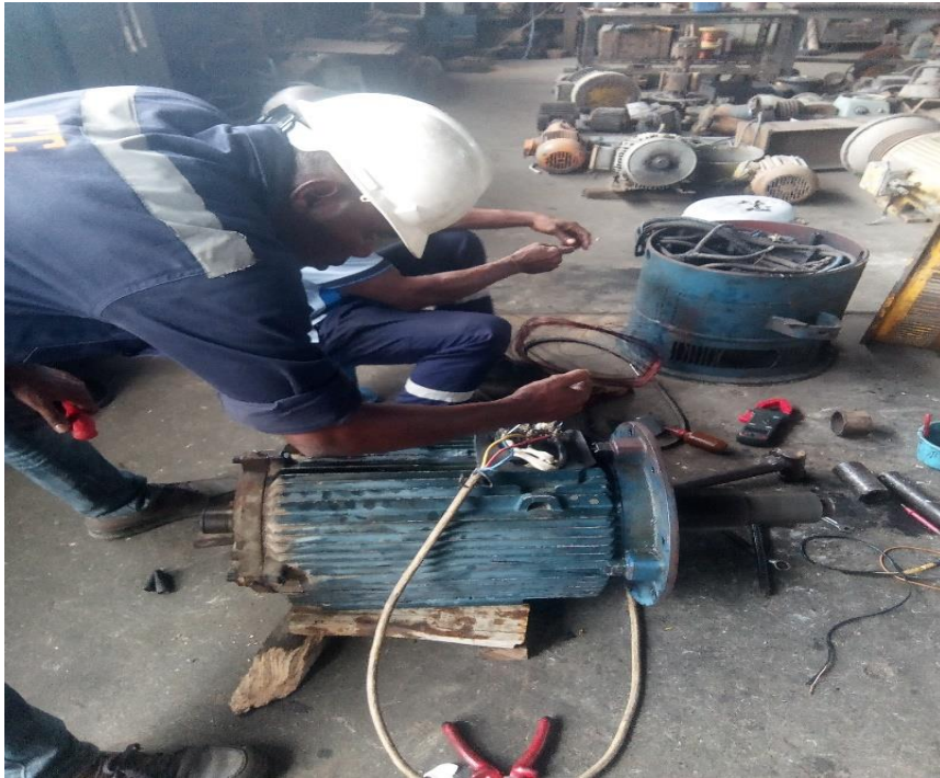
Figure 3: Connection of the 3-phase, 4mm cable to test run the Motor.
