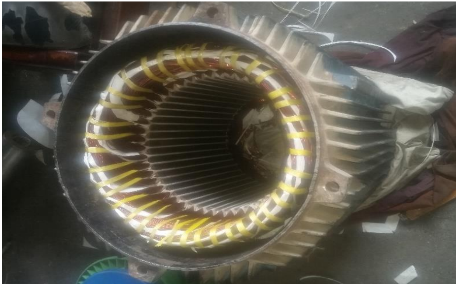
Figure 2: Rewinding completed for a 3-phase. 6HP, 415V, 50Hz Electric Motor.
