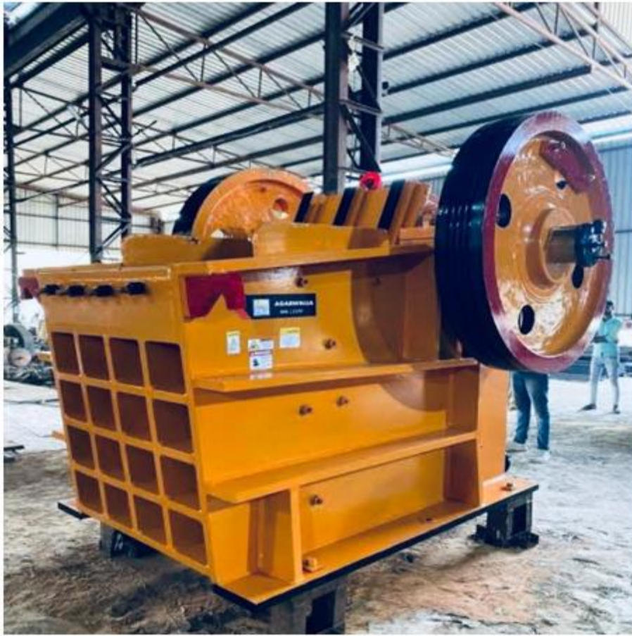
Fig. 7. Structure of a jaw crusher
