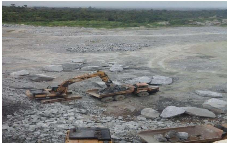
Plate 3.6a: An excavator loading a dump truck at the pit
