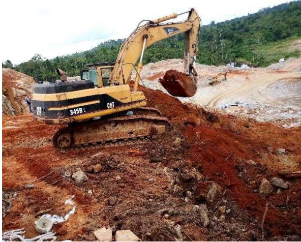
Figure 3.3a: Stripping of Overburden
