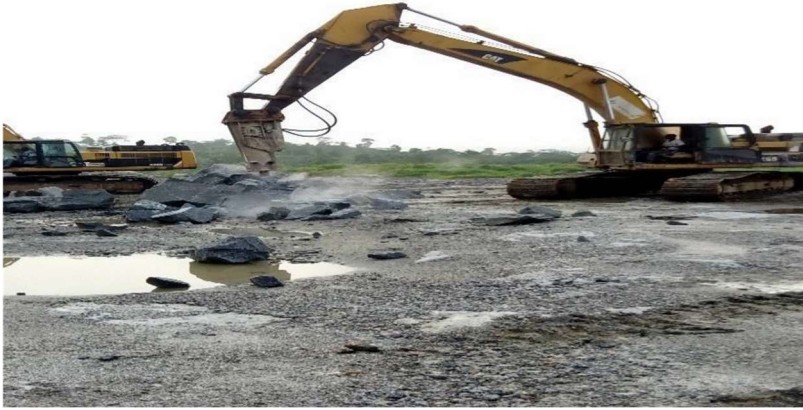
Plate 3.5f: rock breaker performing secondary blasting
