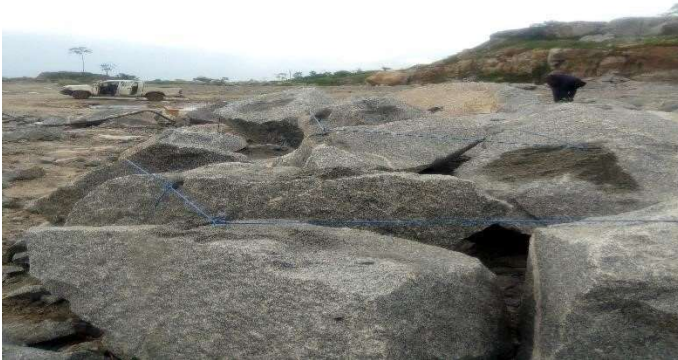
Figure 3.5e: connected boulders with aid of explosive for secondary blasting
