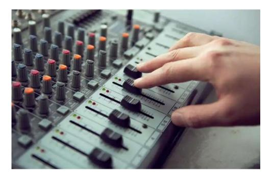
There are analog audio consoles and digital audio consoles, but radio consoles, in general, are specifically designed to be easy for on-air talent to use. In an analog console, the physical audio is actually transmitted through its circuitry. In contrast, digital audio consoles function as a "remote control" for the mix engine (typically located within the rack room).
