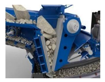
Crushing is the process of reducing the size of solid bodies by breaking them with the aid of external forces, as results of which internal adhesional forces joining the separate particles of the solid body are overcome and new surface are exposed.
