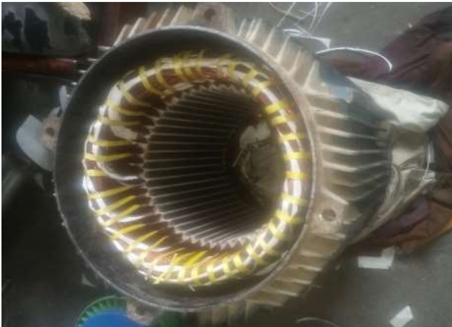
Rewinding completed for a 3-phase. 6HP, 415V, 50Hz Electric Motor.
