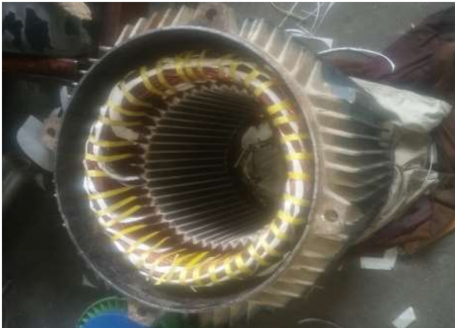
Rewinding completed for a 3-phase. 6HP, 415V, 50Hz Electric Motor.
