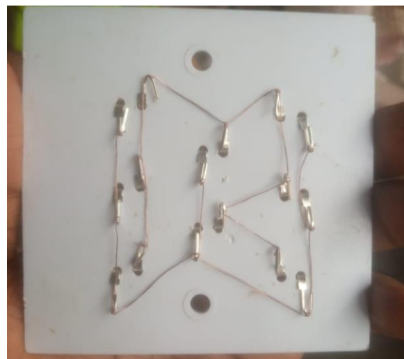
Connection of 5mm Led Bulb with Naked Wire
