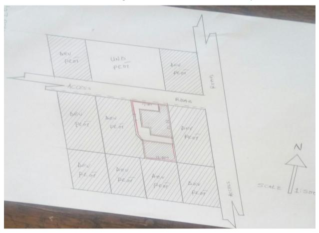
NOTE: The red lines on the sketch shows the boundaries of the main area of observation and the hatched areas signifies build-up plots as of the time of the inspection.
