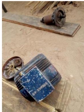
AC Motor Stator with Cover containing bearings and fan
