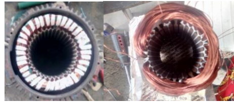
Motor Stator (Field) before and after rewinding
