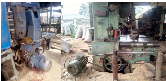
Fig. 8: AC Motors used in band-saw machines
