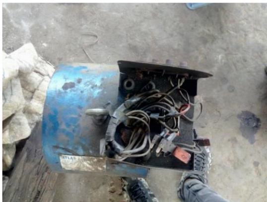
Fig. 10: An Alternator Stator containing Field windings and brushes
