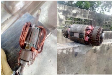
An Armature before and after rewinding
