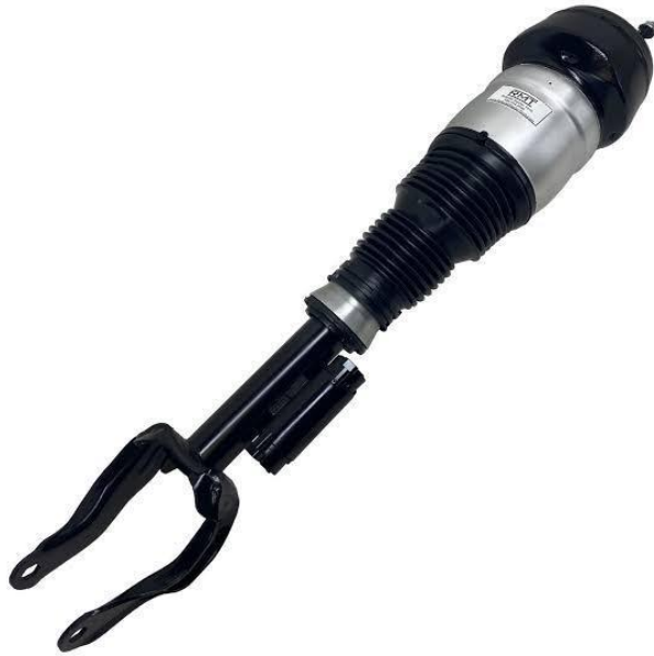
Fig. 3.2: Image of an Airmatic (Balloon) shock absorber
