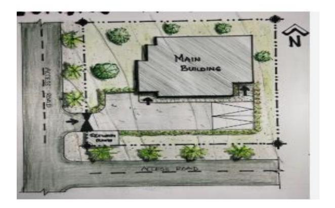
✓ **Site Plan:** A site plan is a drawing that shows what will be built on a piece of land, including any existing improvements. It's also known as a plot plan.
