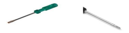
4. Tester: used for testing the positive or availability of supply in the cable.
