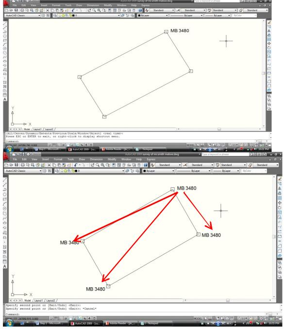
Step 7i: Edit newly copied beacon numbers by double clicking on each, Step 7ii correct the beacon number, MB 3481, MB 3482, MB 3483. *Ok.*
