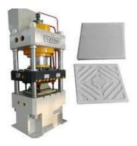
Use: Compresses raw materials to form tiles, ensuring uniform thickness and density.
