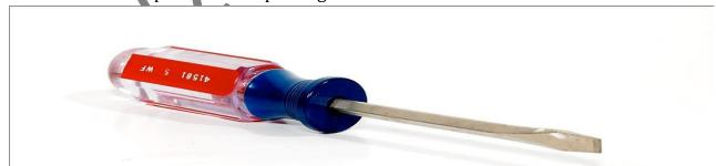
**TESTER:** it is a tool used to detect the flow of current in the system or in a cable and it comprises of three components inside which are the bulb, insulators and lead.
