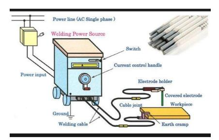
Arc welding is a welding process that uses an electric arc to create enough heat to melt metal, it cools and results in bonding. This fusion welding uses AC or DC power supply as its source of heat. The power supply creates an arc between a consumable or non-consumable electrode, passing either AC or DC current to the base material.
