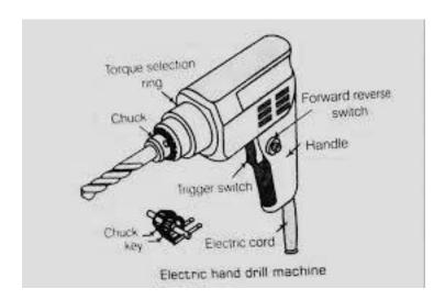
Drill is a tool used for making round holes or driving fasteners. It is fitted with a bit, either a drill or driver chuck. with hand-operated types dramatically decreasing in popularity and cordless battery-powered ones proliferating.
