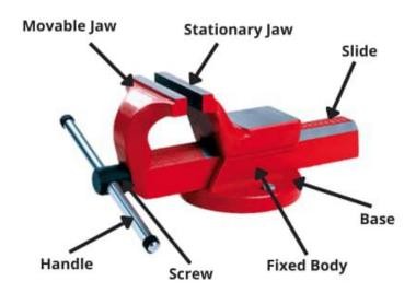
A bench vice, also known as a workshop vice, is a mechanical device designed to hold workpieces firmly in place while performing tasks such as cutting, drilling, filing, or soldering. Typically mounted on a workbench or table, bench vices consist of two jaws – one fixed and one movable – operated by a screw mechanism. This design allows users to adjust the vice to accommodate different workpiece sizes and shapes securely
