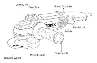
An angle grinder is a handheld power tool that can be used for a variety of metal fabrication jobs that include cutting, grinding, finishing and polishing. The most common types of angle grinders are powered by electricity; either corded or battery powered.
