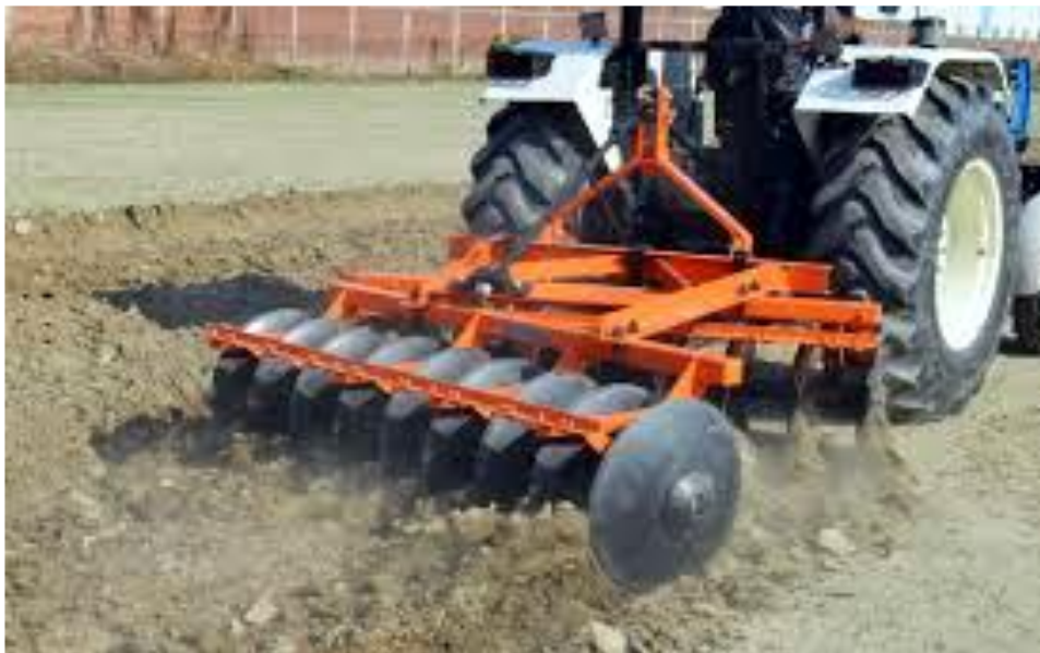
THE DISC HARROW MOUNTED TO TRACTOR AFTER THE REPAIR
