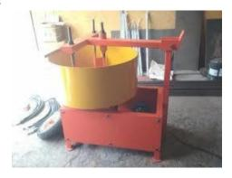
**Use**: Combines raw materials (clay, sand, pigments) to create a consistent mixture for tile production.
